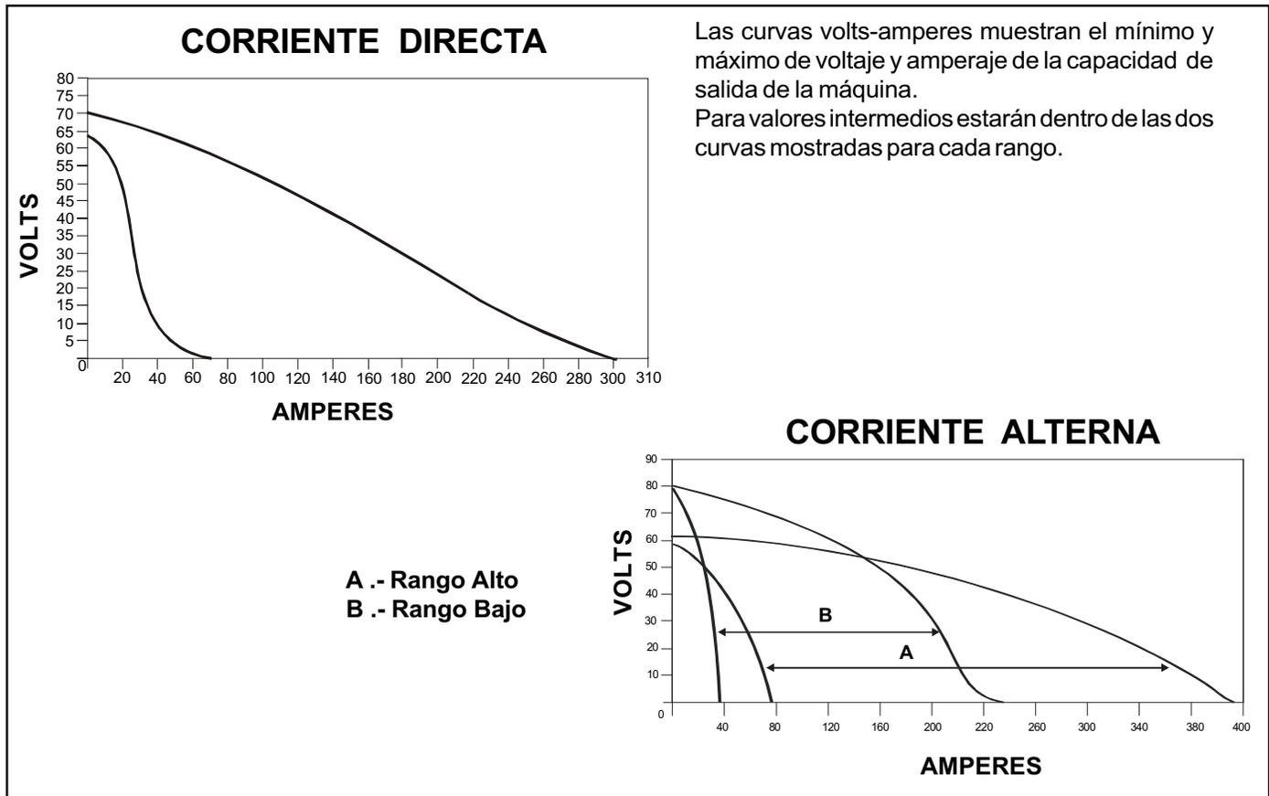
FIGURA 2-1 CURVAS VOLTS-AMPERES.
