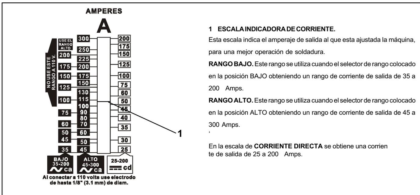
FIGURA 4-4 ESCALA INDICADORA DE CORRIENTE.
